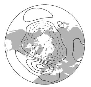
Figure 3. Geopotential height  $\Phi_{1000}$  anomalies in each of the three winter months (JFM) for all the runs (LABMAX, CTRL, LABMIN) regressed onto the NAO<sub>m</sub> index (see text for further explanation). Contour interval is 10 m, positive (solid) and negative (dashed). The zero line is omitted
